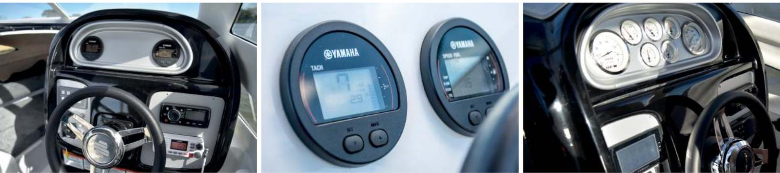
We have found that it is not uncommon for instruments to develop a certain amount of condensation under the glass. This is often the result of atmospheric or storage conditions and will usually disappear over a short time. The condensation will not interfere with the function of the gauge and replaced gauges will possibly still do the same.
